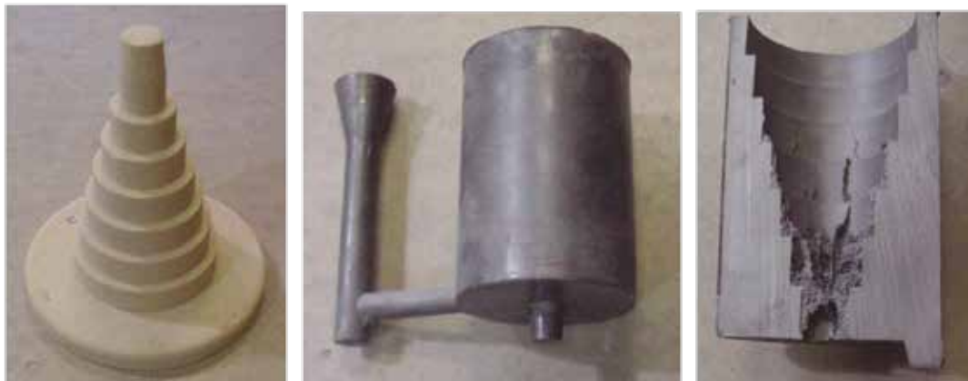
Figure 2. The stepcone core (left), casting (center), and sectioned casting (right) are shown above.
