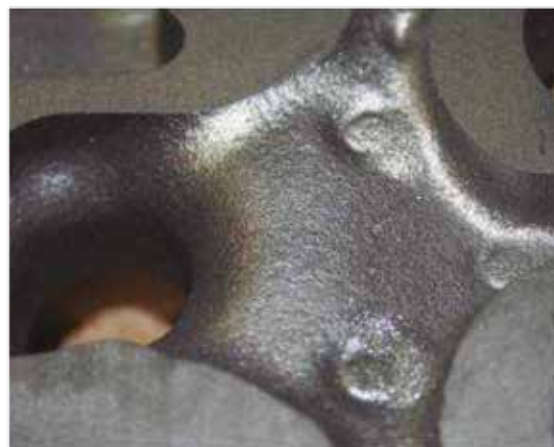
Figure 7. Casting surface with MIRATEC TS
