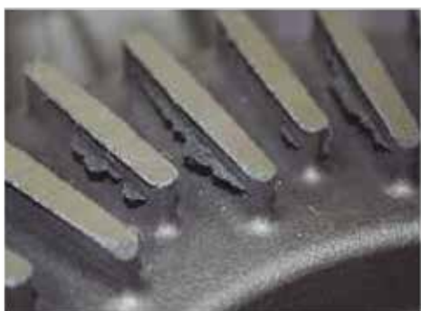
Figure 4. Break disk with veining
