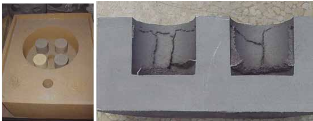
Figure 3. The 2x2 cores and mold (left) and a sectioned casting (right) exhibiting the veining defect are shown above.
